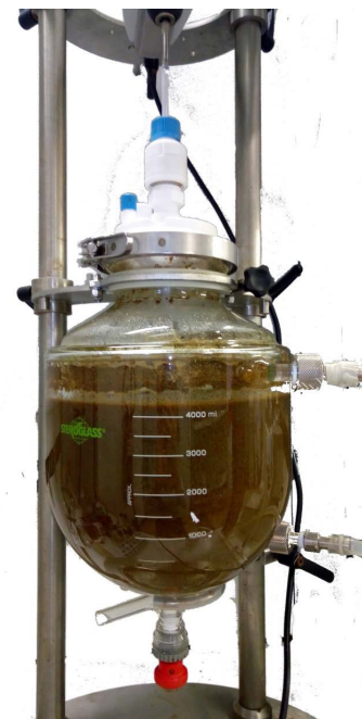
Lab-scale set-up for EAE of coffee green beans at Uni Parma
